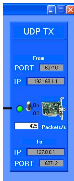
Figure 2.5-7 UDP Tx part of the HO analyser user interface
