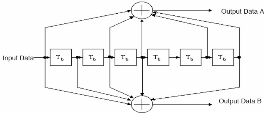
Figure 3 Convolutional encoder with constraint length 7
