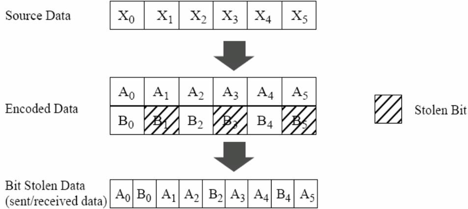
Figure 5 Puncturing of encoded bits for code rate of 2/3
