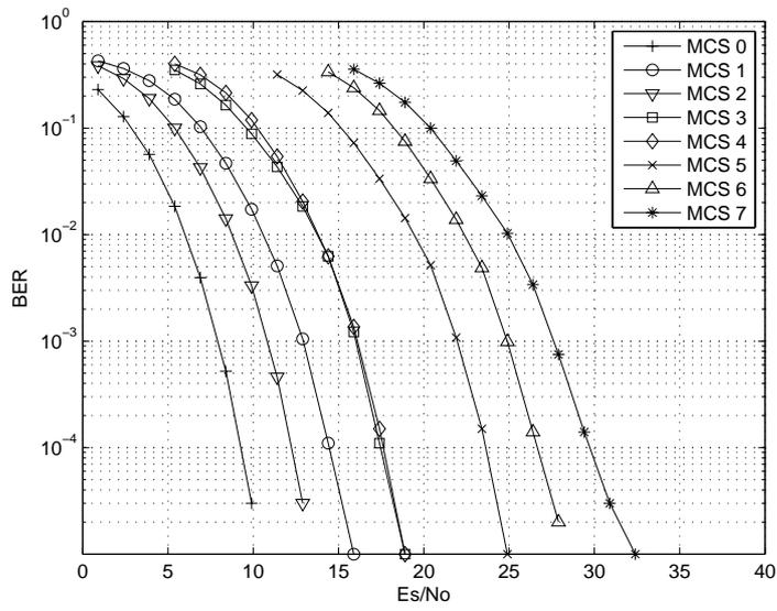
Figure 14 BER of WLAN in Channel D
