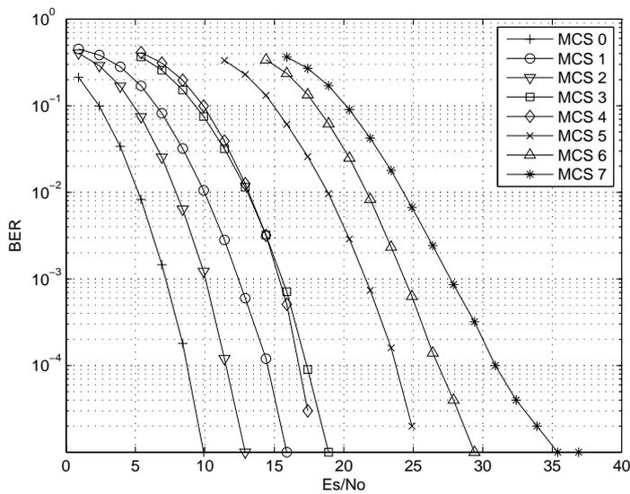
Figure 13 BER of WLAN in Channel C
