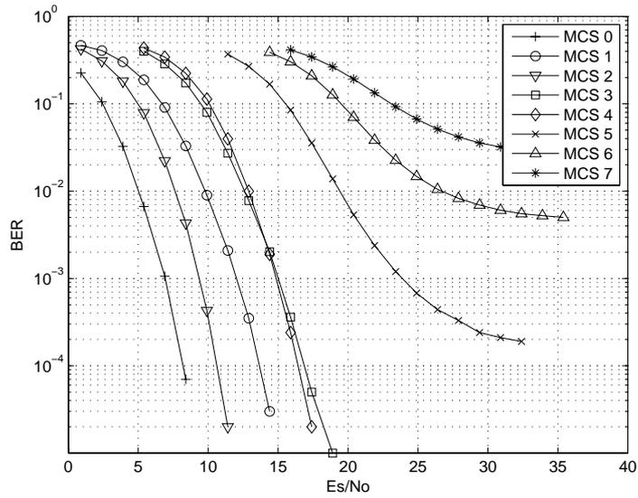
Figure 15 BER of WLAN in Channel E
