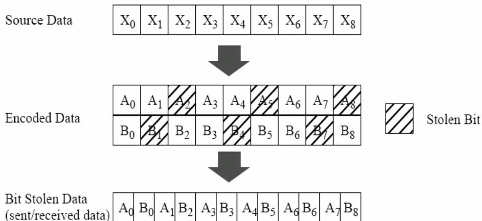
Figure 4 Puncturing of encoded bits for code rate of 3/4
