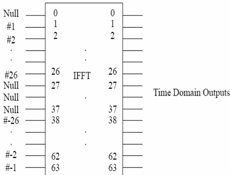
Figure 8 Loading pilot and data symbols onto subcarriers followed by OFDM modulation
