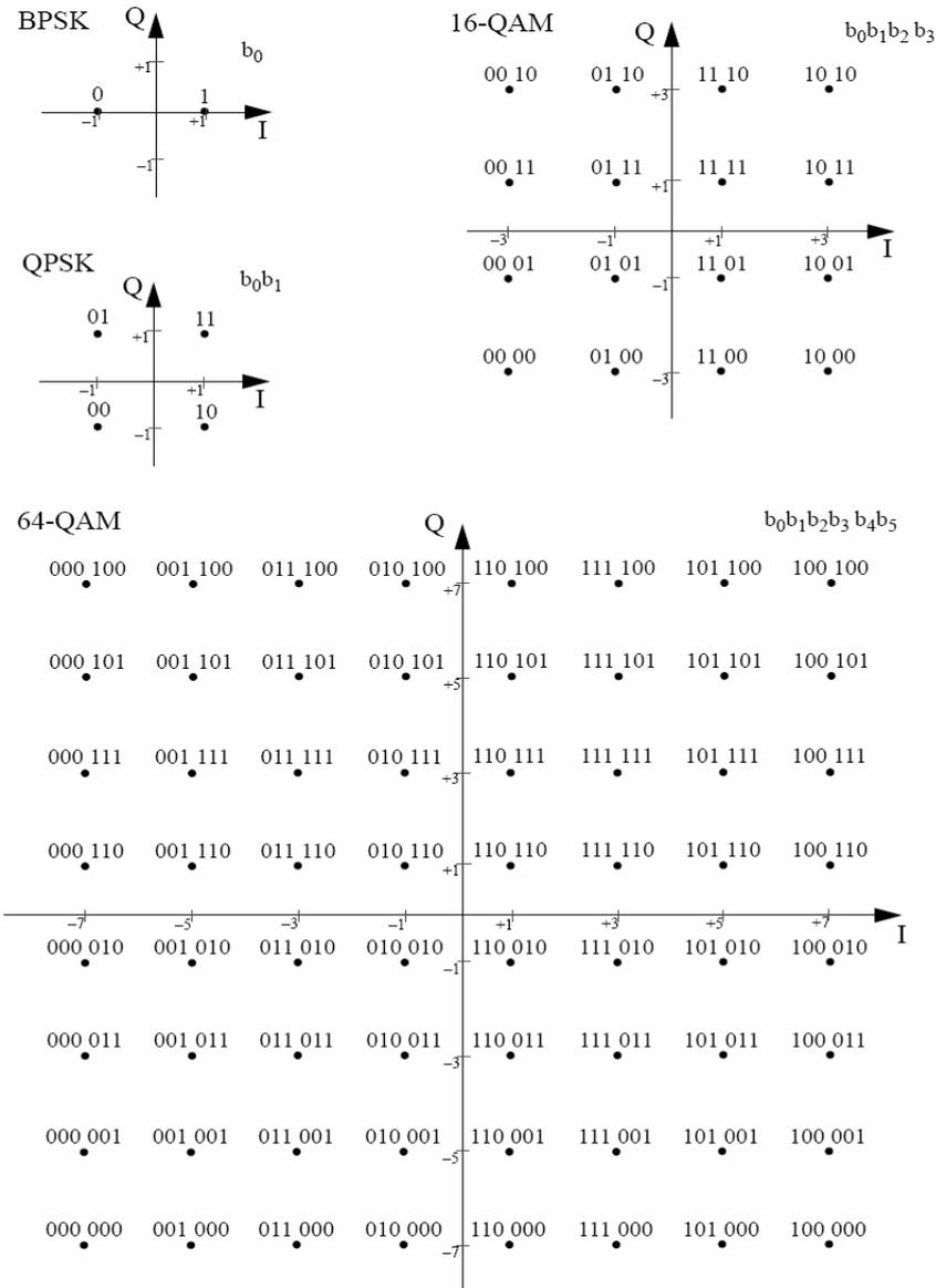
Figure 6 Mapping of serial input bits into complex value
