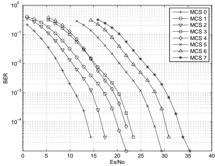
Figure 11 BER of WLAN in Channel A
