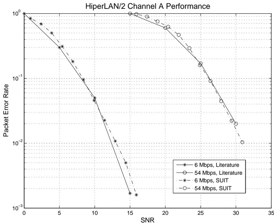
Figure 10 Comparison of the SUIT WLAN simulator to results in the literature
